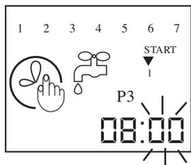
The three arrows under **START** indicate the three different irrigations. As each arrow appears you may program the start time for that particular irrigation.
