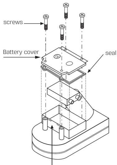
When replacing the seal, push seal tabs into slots.
